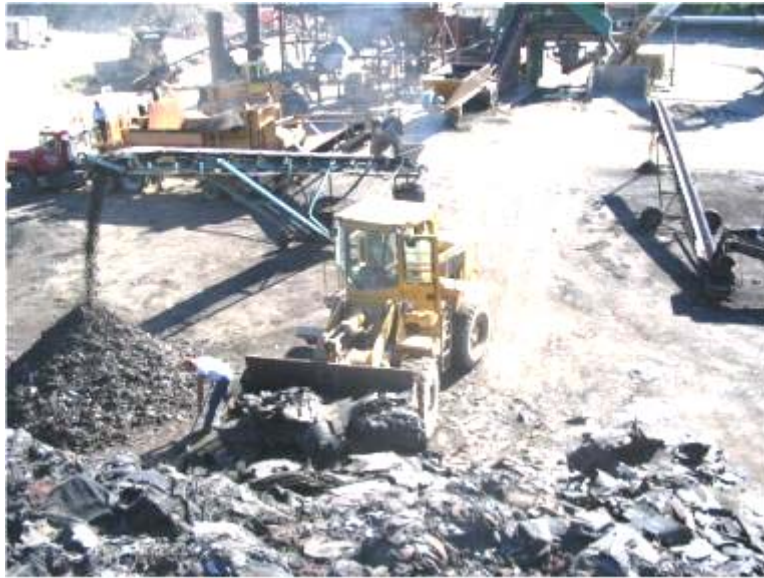
Picture 12 - Front End Loader and Operator Moving Material from a Pile of Source Separated Tear-Off Shingles
