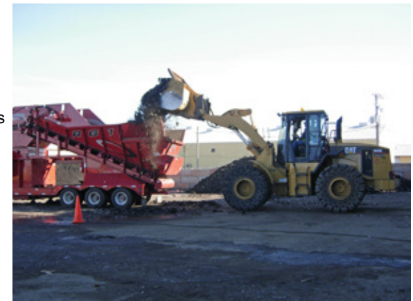
A Caterpillar 950G wheel loader scoops used shingles into the hopper which force feeds them into a rotor to be broken into consistent sizes.
