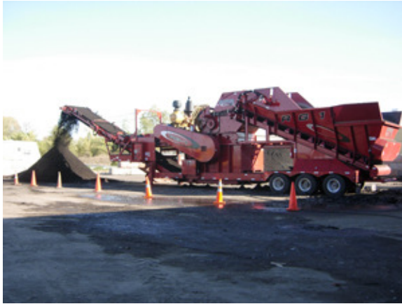
Dem-Con acquired a Rotochopper RG1 that grinds used asphalt shingles and removes nails and other metals. The ground shingles move on a conveyor belt into a bin.
